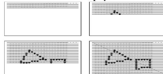
Electron beam traces over screen in **raster scan order**.
