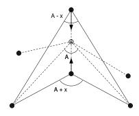
As can be expected, it shows a more stable behavior when returning to the original shape after deformation. However, it constrained the motion of each particle more than necessary, sometimes resulting in almost rigid body-like motions (as can be seen in the third animation sequence of the artifact).
