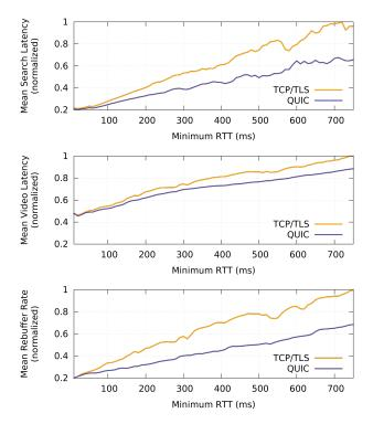
Figure 9: Comparison of  $QUIC_g$  and  $TCP_g$  for various metrics, versus minimum RTT of the connection. The y-axis is normalized against the maximum value in each dataset. Presented data is for desktop, but the same trends hold for mobile as well. The x-axis shows minimum RTTs up to 750 ms, which was chosen as reasonable due to Figure 8: 750 ms encompasses over 95% of RTTs and there is no information gained by showing more data.
