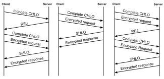
Initial 1-RTT Handshake Successful 0-RTT Handshake Rejected 0-RTT Handshake
