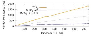
Figure 7: Comparison of handshake latency for  $QUIC_g$  and  $TCP_g$  versus the minimum RTT of the connection. Solid lines indicate the mean handshake latency for all connections, including 0-RTT connections. The dashed line shows the handshake latency for only those  $QUIC_g$  connections that did not achieve a 0-RTT handshake. Data shown is for Desktop connections, mobile connections look similar.
