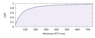
Figure 8: Distribution of connection minimum RTTs for TCP connections to our servers. These results were gathered from video playbacks. The distribution is similar for search connections.
