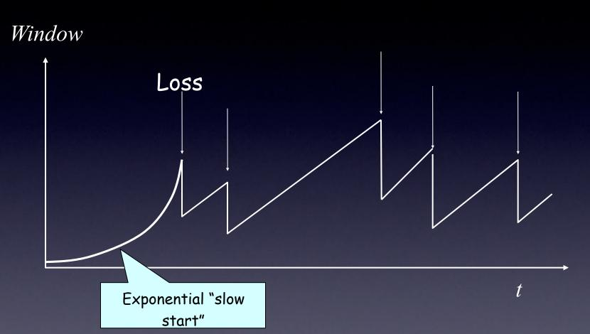
Why is it called slow-start? Because TCP originally had no congestion control mechanism. The source would just start by sending a whole receiver window's worth of data. • Recall that we have fast retransmit
