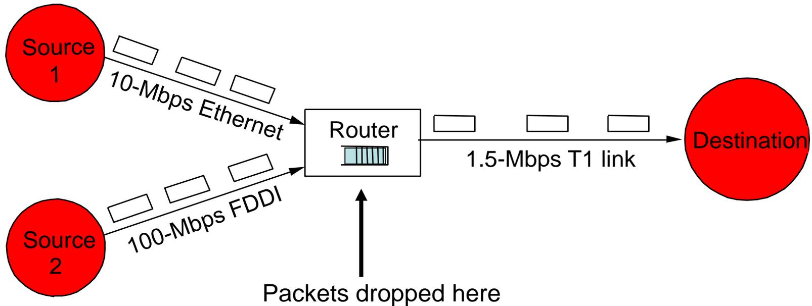
Buffer absorbs bursts when input rate  $>$  output
