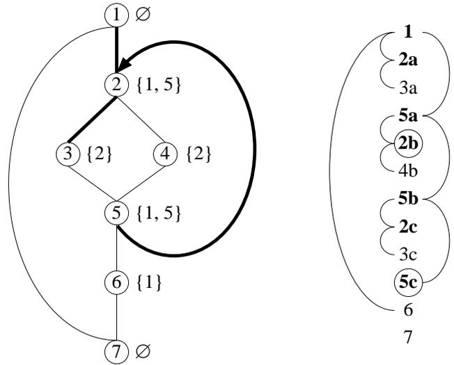
Figure 2: Example Flow Graph and Trace
