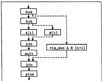
Figure 10: Control graph for concurrent loads and iterations
