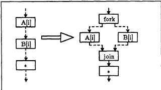
Figure 7: Sequential and parallel control flows for the two loads
