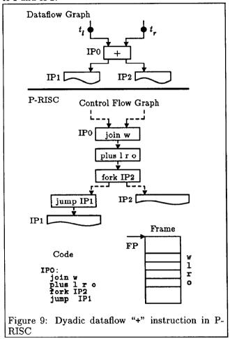
The P-RISC control graph is shown next, followed by the P-RISC code and frame. The slots 1 and r are used to hold the left and right input values, respectively; the slot o is used to hold the output value, and the slot w is used for synchronization.
