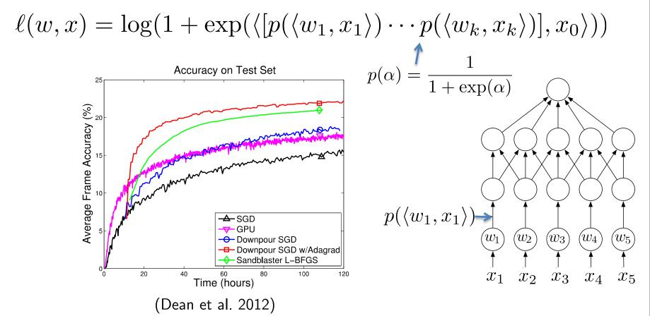
Distributed,  $d = 1.7 \cdot 10^9$  parameters. SGD and AdaGrad use 80 machines (1000 cores), L-BFGS uses 800 (10000 cores)
