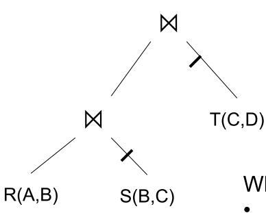
Every operator is a hash-join and implements the iterator model
