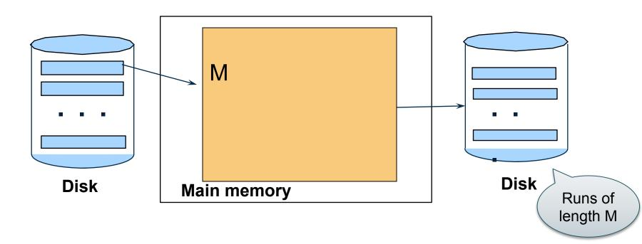
Can increase to length 2M using "replacement selection" (How?)
