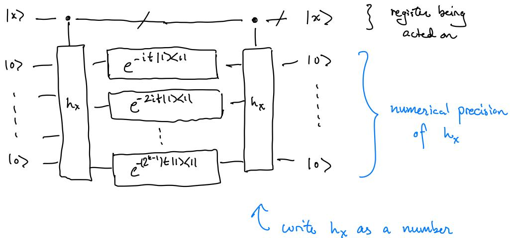
$$\text{If } h_x = h_x^{(0)} + 2h_x^{(1)} + 4h_x^{(2)} + \dots + (2^{k-1})h_x^{(k-1)}$$
