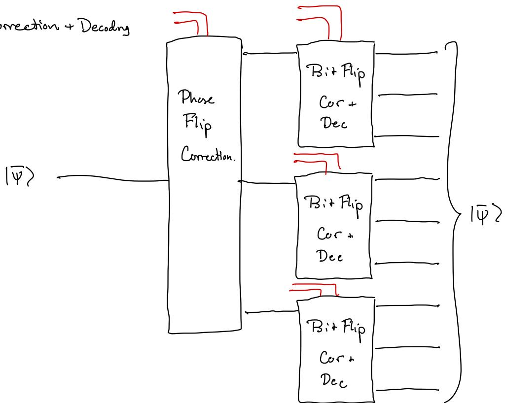
This corrects any 1 bit flip error per triple and 1 phase flip error. To correct bit + phase flip error in the same qubit, both syndromes check.
