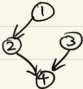
$$I(G) = \left\{ \begin{array}{l} X_3 \perp\!\!\!\perp (X_1, X_2) \\ X_1 \perp\!\!\!\perp X_4 \mid (X_2, X_3) \end{array} \right\}$$
