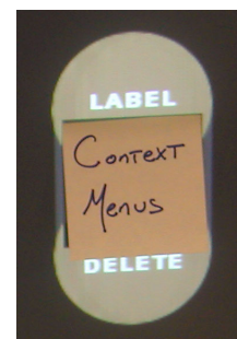
Figure 5. Tapping on a note invokes an electronic context menu for physical content.
