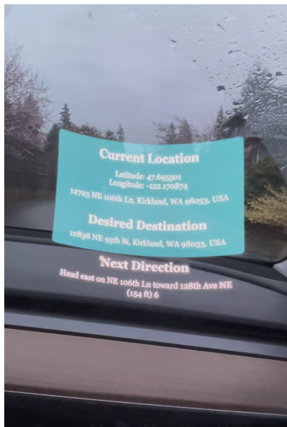
Fig. 1. [See teaser demo video in folder]. Visual of the AR application while driving, displaying current location, destination, and the next direction to take.
