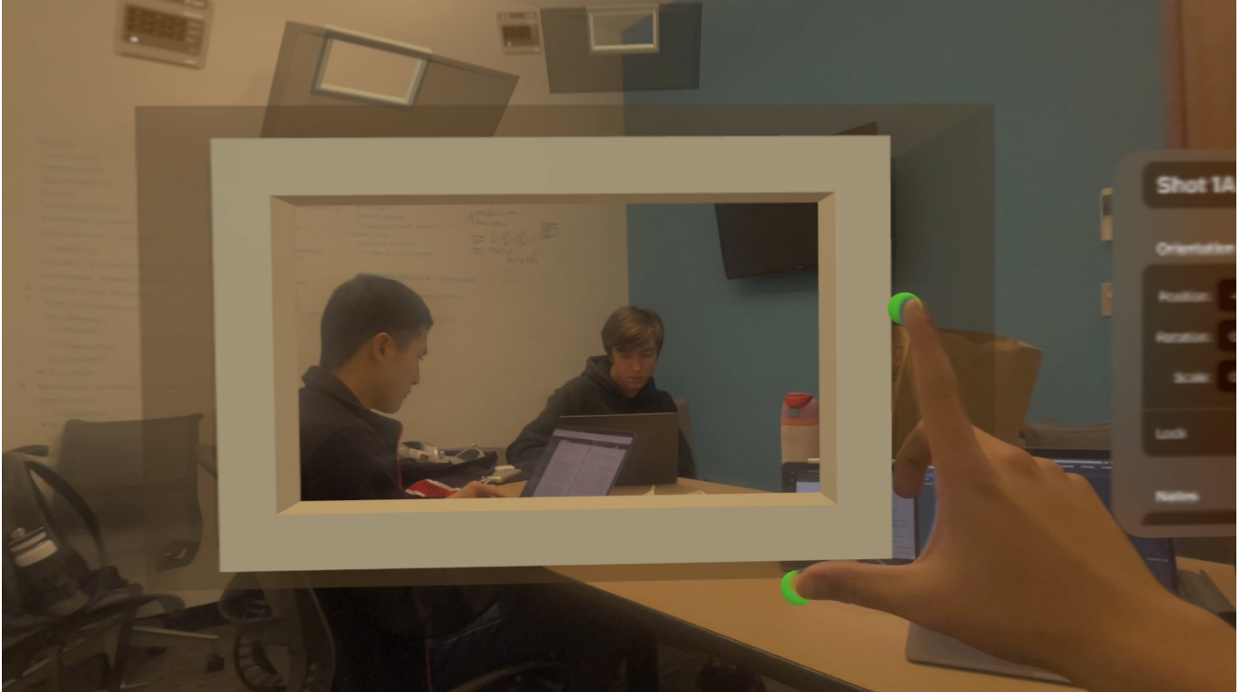
Fig. 1. A user of StoryboardXR adds a frame to their view using the hand gesture, planning for a shot in the scene.
