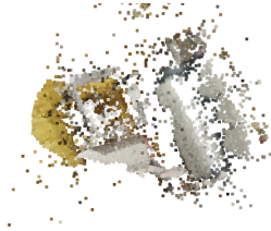
Fig. 11. Dense point cloud associated with a empty table (notice how there are no blue or gray objects on the table's surface)
