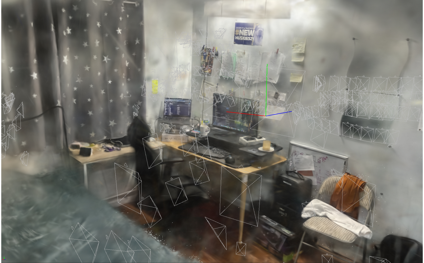
Fig. 1. This is a sample gaussian splat of Derek’s bedroom. The structure from motion (SFM) metadata including camera field of views and image clips. This represents the software side of our pipeline, which will be explored more later in the paper.
