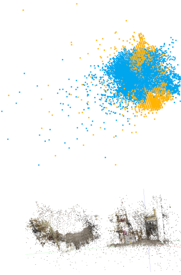
Fig. 3. Results of merging two corners of a room using Open3D's global registration. The bottom images show the original point clouds, while the top images illustrate the voxelized point clouds after merging.
