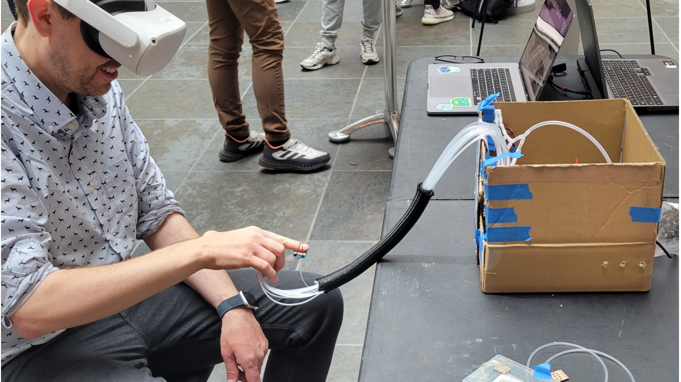
Fig. 1. A small haptic device attached to the index finger of a users. This device is capable of applying pressure at varying locations on the fingerpad via inflating bubbles. When interacting with objects in a virtual environment, this localized pressure can be used to mimic the sensation of real touch.
