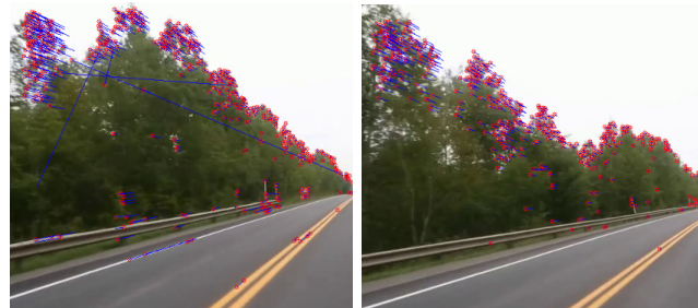
Matching before RANSAC Matching after RANSAC (red dots are extracted keypoints and blue lines shows the movements of keypoints between frames)
