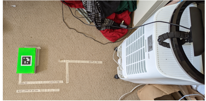
Fig. 4. The webcam can be seen at the right, looking down at the box, which is placed at the origin in this image.
