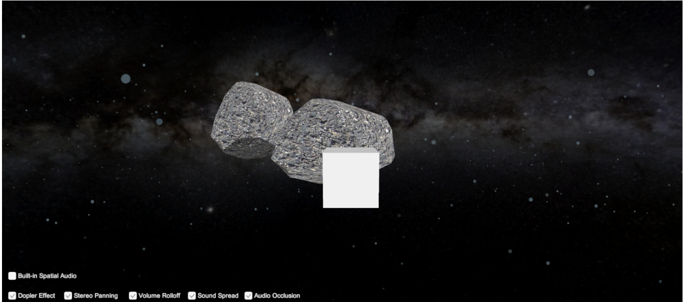
Fig. 1. This screenshot depicts a scene where a cube serves as the sound source. The cube can be repositioned in various directions, including the z-axis, which alters the perception of the sound. Additionally, the user has the ability to adjust the yaw rotation of the camera using their head position, further influencing the perception of the sound.
