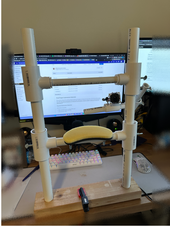
Fig. 2. Adjustable head-chin rest with camera setup. The head rest, chin rest, and camera positions are adjustable for different users and conditions.
