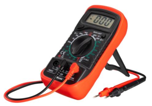
A multimeter is a tool that measures how much electricity is in a circuit. Most multimeters show the measurements on a screen that blind people can't see. There are talking multimeters for sale but they can be expensive. There are instructions to build at talking multimeter yourself<sup>8</sup>.
