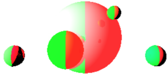
Fig. 2. The re-projected right-eye image with modified colors to show the re-projection algorithm in action. The green pixels, as well as most of the white space, have been re-projected. Only the red regions required re-tracing.
