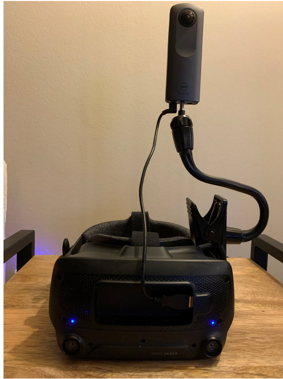
Fig. 1. A Valve Index HMD connected to a PC displayed an FOV-compressed view of the live video provided by the Ricoh Theta V 360° camera. The camera was connected to the PC via the Index's "frunk."
