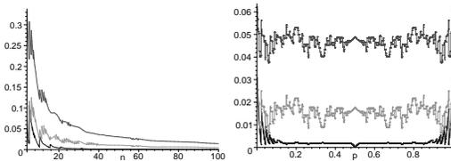
Average redundancy rates of Gilbert-Moore, Shannon, and Huffman block codes (left: fixed source  $\Pr(0) = 1/8$ ; right: fixed block  $n = 32$ ,  $p = \Pr(0)$ ).
