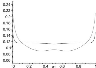
Redundancy rates of block universal codes under a binary source with  $\Pr(0) = p$ . Block size  $n = 32$ .
