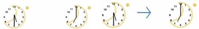
Figure 4. Ambiguity in iconic representation due to cultural biases: Our initial design indicating start and end times for a job places the start time at left (left). This is misinterpreted in Muslim culture. Adding an arrow avoids this problem (right).
