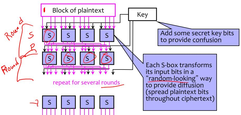
Block of ciphertext
