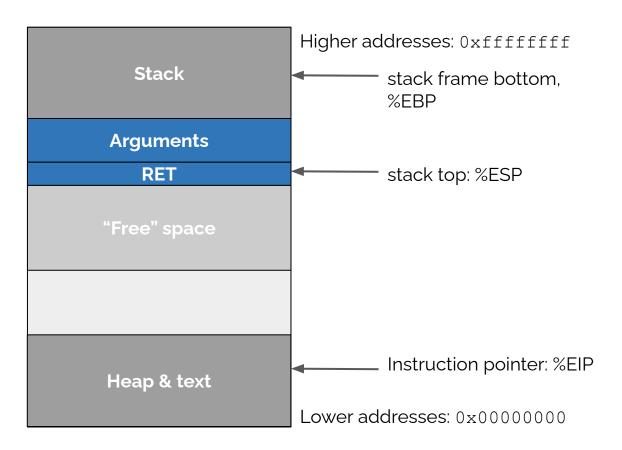
Higher addresses: 0xffffffff Stack stack frame bottom. %EBP **Arguments** stack top: %ESP Instruction pointer: %EIP Heap & text Lower addresses: 0x00000000
