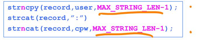
MAX\_STRING\_LEN bytes allocated for record buffer
