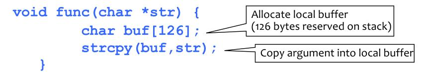
When this function is invoked, a new frame (activation record) is pushed onto the stack.
