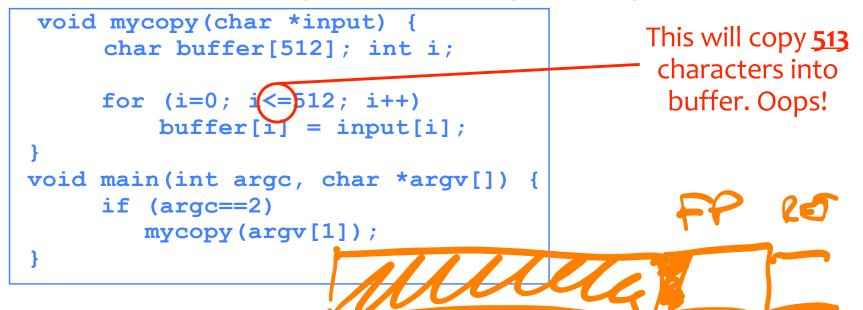
1-byte overflow: can't change RET, but can change pointer to previous stack frame...
