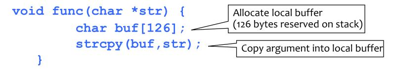
• When this function is invoked, a new frame (activation record) is pushed onto the stack.
