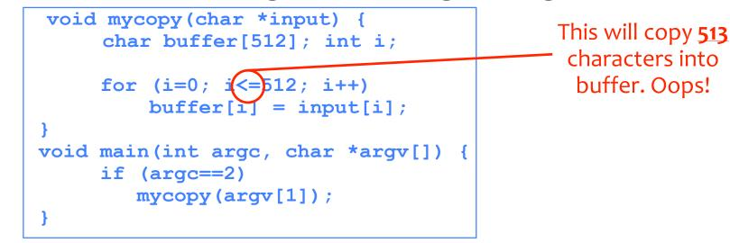
1-byte overflow: can't change RET, but can change pointer to previous stack frame...
