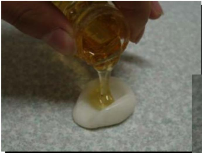
**Pour the liquid into the mold.**
