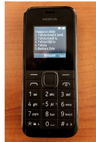
Figure 2. eKichabi main menu accessed via USSD on a demo handset from the Phase 1 focus groups.
