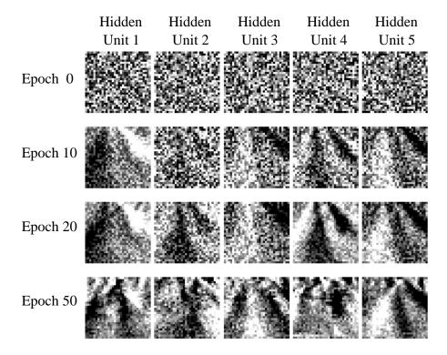
Figure 5: The weights projecting from the input retina to the 5 hidden units in an ALVINN network at four points during training on a lined two-lane highway. Black squares represent inhibitory weights and white square represent excitatory weights. The diagonal black and white bands on weights represent detectors for the yellow line down the center and the white line down the right edge of the road.
