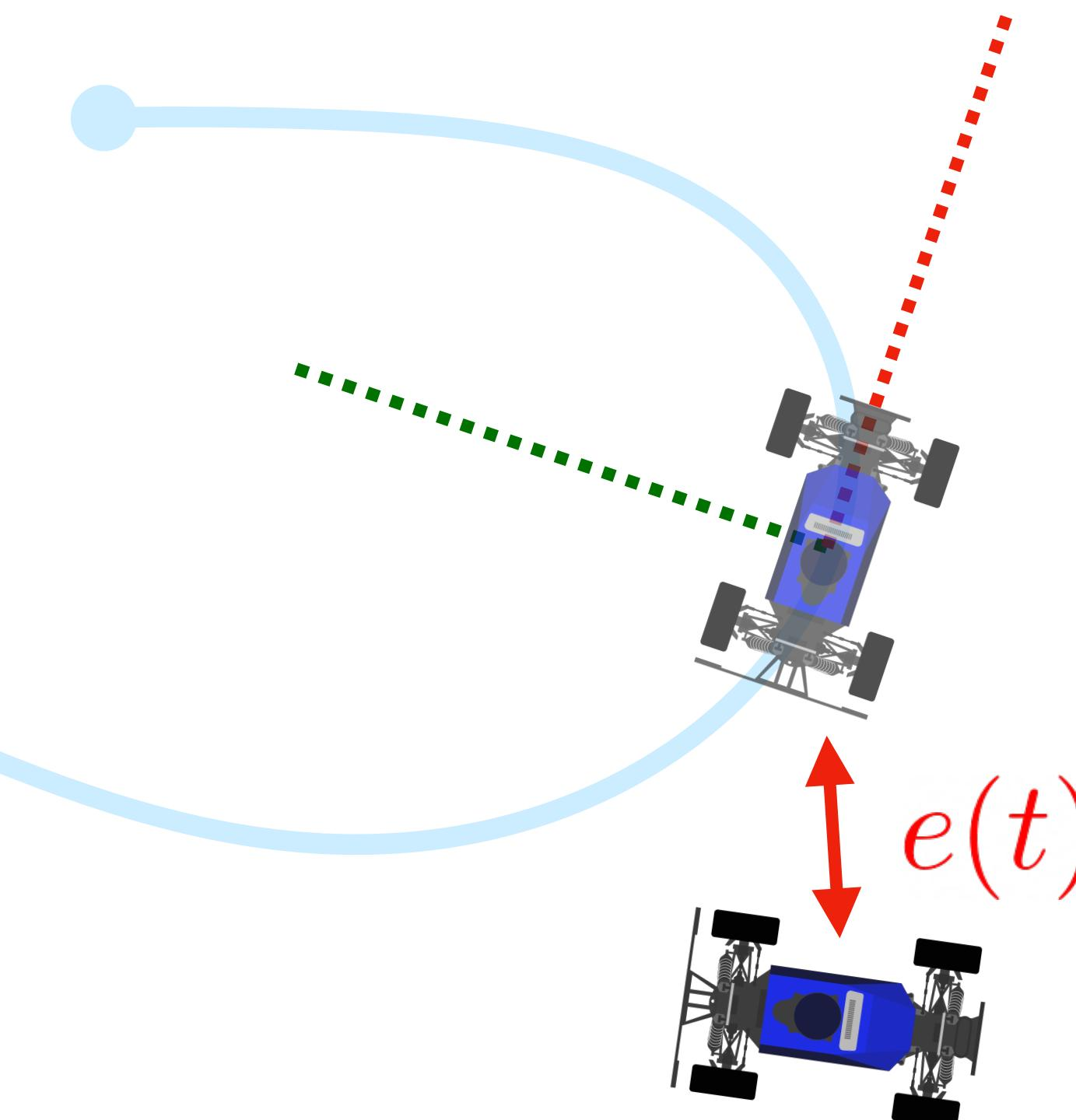
The diagram illustrates the computation of error to a reference state. A blue dashed line represents a circular track. A green dashed line extends from the center of the track to a blue racing car. A red double-headed vertical arrow labeled  $e(t)$  indicates the vertical displacement of the vehicle from the track center. A second blue racing car is shown on the track, representing the reference state.
