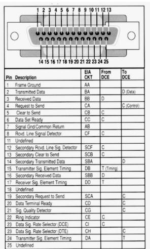
Fig.6. RS232 DB25 connector
