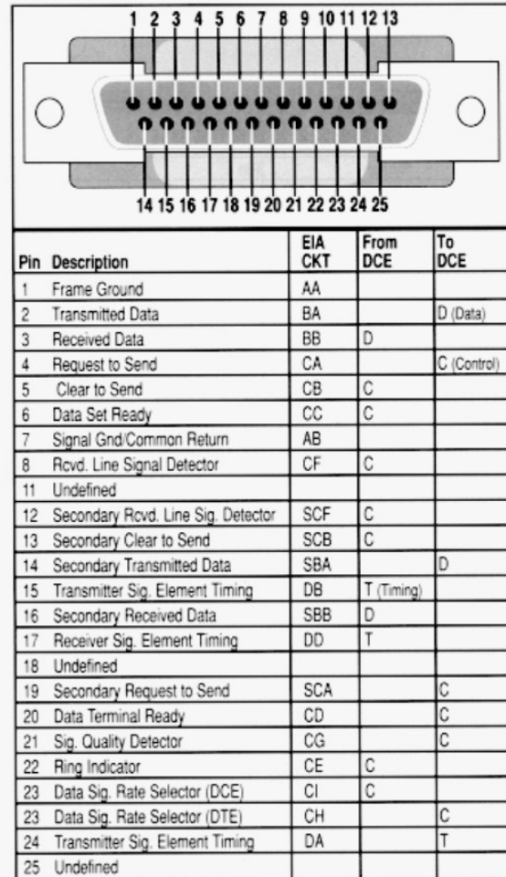
Fig.6. RS232 DB25 connector
