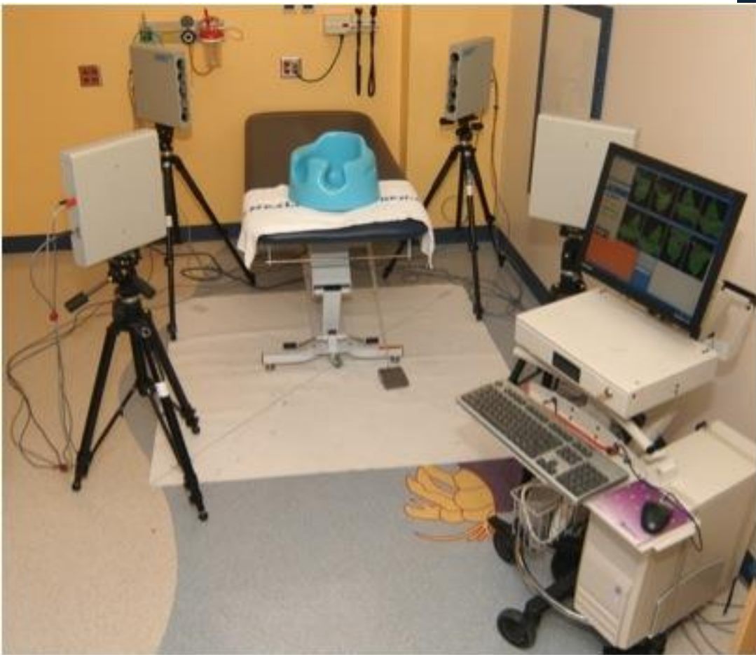
3dMD multi-camera stereo system
