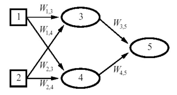
Feed-forward network = a parameterized family of nonlinear functions:
