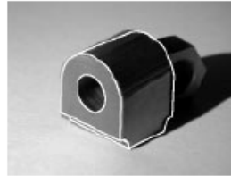
Figure 18: The pose computed from six point correspondence using the algorithm described in Section 5.2.
