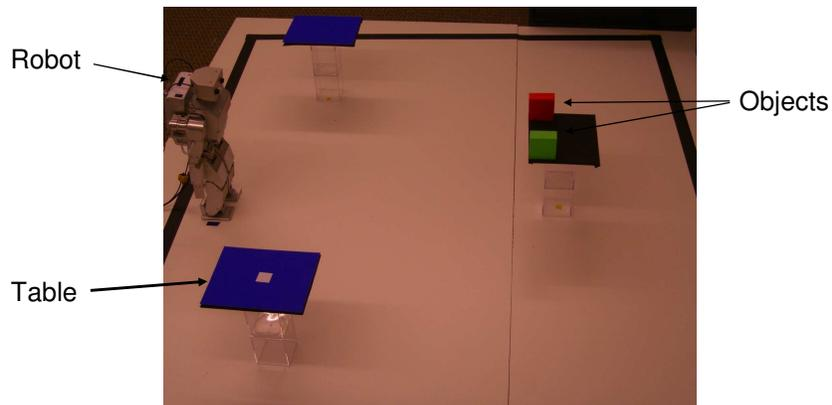
**Task:** Use brain signals to command robot to fetch red (or green) object and bring it to one of the tables.
