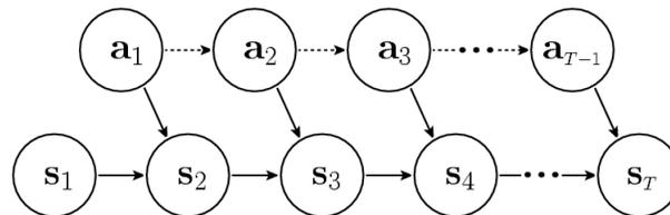
**Infer actions  $a_t$  given evidence  $s_1, \dots, s_T$  from teacher subject to stability constraints on gyro readings**
