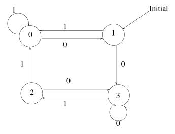
States are labelled 0, 1, 2, 3. Transitions are indicated by the arrows and occur everytime the input in is assigned a value of either 0 or 1.
