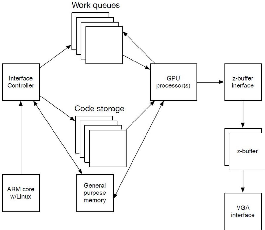
Figure 1: Rough System Diagram of GPU
