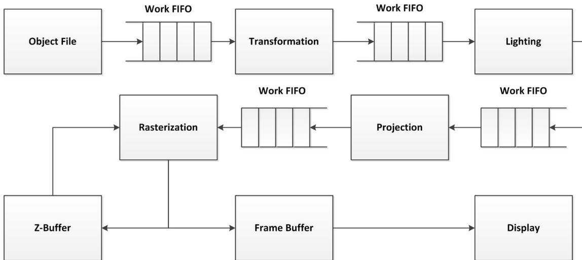
Figure 2: High level graphics pipeline
