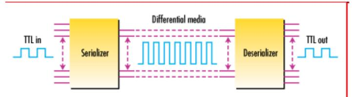
▲ Serdes technology is based on a serializer/deserializer pair where typical inputs, TTL signals (0 to 3.3-V swing) enter the serializer 'horizontally' and are then 'vertically' aligned so that in one clock period one set of parallel bits, or just one word, is transmitted. The internal frequency of the serializer must be faster than the incoming TTL data.
