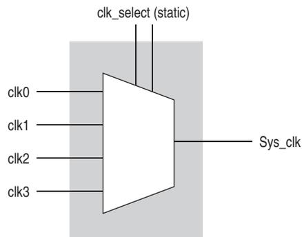
The datasheet for your target device describes how LUT outputs may glitch during a simultaneous toggle of input signals, independent of the LUT function. Although in practice the 4:1 MUX function does not generate detectable glitches during simultaneous data input toggles, it is possible to construct cell implementations that do exhibit significant glitches, so this simple clock mux structure is not recommended. An additional problem with this implementation is that the output behaves
