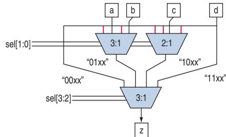
Implementing this version of the multiplexer still requires at least five 4-input LUTs, two for each of the remaining 3:1 multiplexers and one for the 2:1 multiplexer. This design selects an output from only four inputs, a 4:1 binary multiplexer can be implemented optimally in two LUTs, so this degenerate multiplexer tree reduces the efficiency of the logic.
