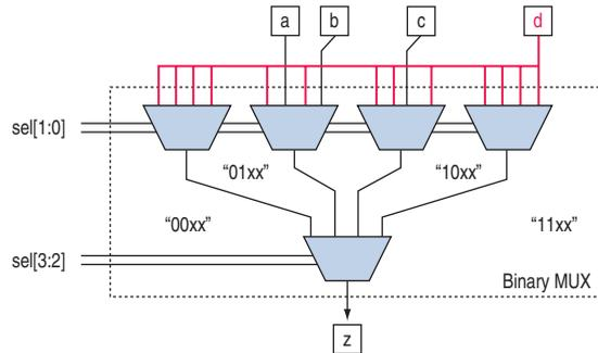
In the example in [Figure 6–6](#), the first and fourth multiplexers in the top level can easily be eliminated because all four inputs to each multiplexer are the same value, and the number of inputs to the other multiplexers can be reduced, as shown in [Figure 6–7](#).
