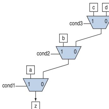
An  $N$ -input priority multiplexer uses a LUT for every 2:1 multiplexer in the chain, requiring  $N - 1$  LUTs. This chain of multiplexers generally increases delay because the critical path through the logic traverses every multiplexer in the chain.
