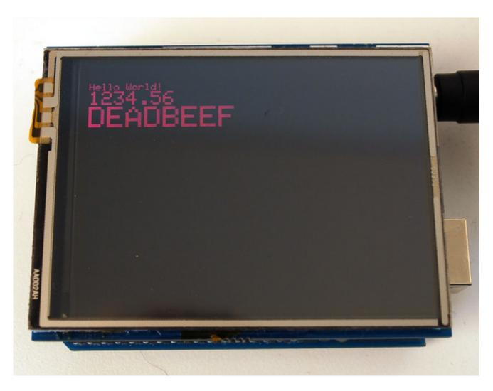
After setting everything up, you can use print() or println() — *just like you do with Serial printing!* For example, to print a string, use print("Hello world") - that's the first line of the image above. You can also use print() for numbers and variables — the second line above is the output ofprint(1234.56) and the third line is print(0xDEADBEEF, HEX).
