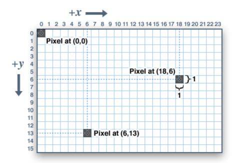
Coordinates are always expressed in pixel units; there is no implicit scale to a real-world measure like millimeters or inches, and the size of a displayed graphic will be a function of that specific display's *dot pitch* or pixel density. If you're aiming for a real-world dimension, you'll need to scale your coordinates to suit. Dot pitch can often be found in the device datasheet, or by measuring the screen width and dividing the number of pixels across by this measurement.
