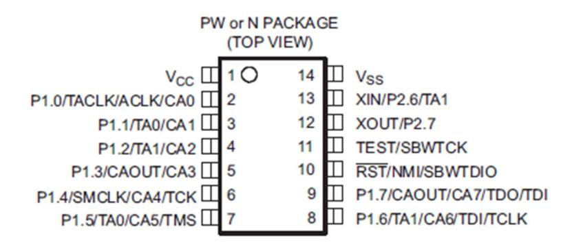
PWM can be configured to appear on TA1 pins PxSEL.x that chooses which pin TA1 connects to
