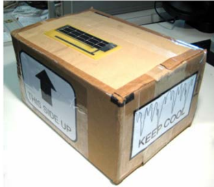
Figure 9. Passive solar antenna-based data logger on a parcel.
