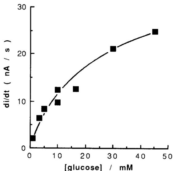
Fig. 3. The dependence of the initial value of  $di/dt$  on the glucose concentration for additions of glucose oxidase (500 ng) to the cell at a potential of 0.4 V.
