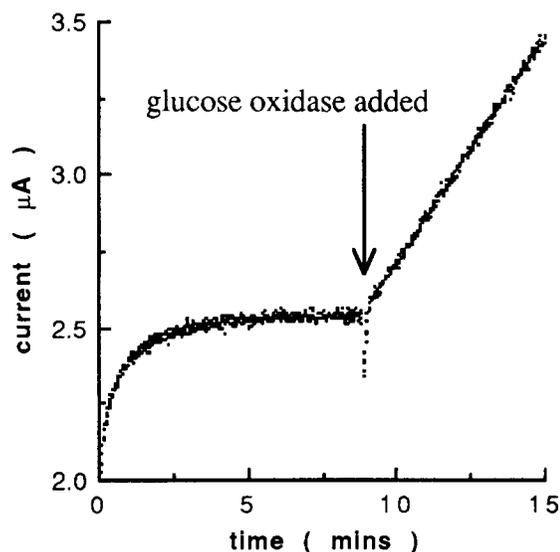
Fig. 5. Amperometric response to addition of glucose oxidase (100 ng) over a short time scale (polarizing potential, 0.4 V; glucose concentration, 30 mM; the final concentration of glucose oxidase in the cell was 0.317 nM).
