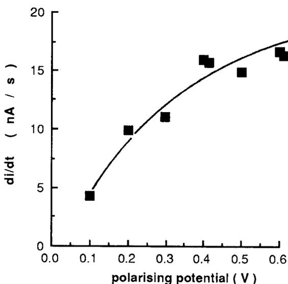
Fig. 2. The dependence of the initial value of  $di/dt$  on the potential for the addition of glucose oxidase (500 ng, 1 nM; 3.04 ml cell volume; glucose concentration, 9.9 mM).
