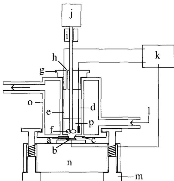
Fig. 1. Schematic diagram of the apparatus with the cell drawn to the scale shown. (a), working electrode; (b), platinum disc contact; (c), silicone rubber gasket; (d), platinum counter electrode; (e), Ag/AgCl reference electrode; (f), glass propeller; (g), PTFE stopper; (h), injection port; (i), PTFE collar; (j), motor; (k), potentiostat; (l), water from constant temperature bath; (m), sprung catch to hold cell onto base; (n), perspex base; (o), glass cell; (p), electrolyte.
