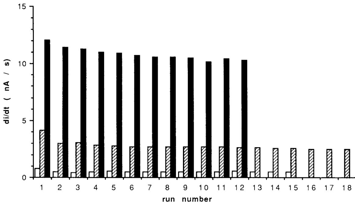
Fig. 7. The reproducibility of the standard procedure used to determine  $di/dt$  (glucose oxidase concentration in the cell, 0.063 (□), 0.317 (▨), 1.59 nM (■); polarizing potential, 0.4 V; glucose concentration, 30 mM).
