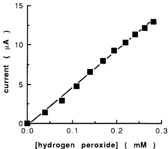
Fig. 8. The dependence of the steady state current for the oxidation of hydrogen peroxide on the bulk hydrogen peroxide concentration (polarizing potential, 0.4 V; glucose concentration, 30 mM).
