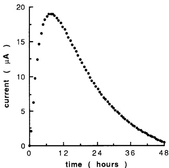
Fig. 4. Amperometric response to addition of glucose oxidase (100 ng) over a long time scale (polarizing potential, 0.4 V; glucose concentration, 30 mM).
