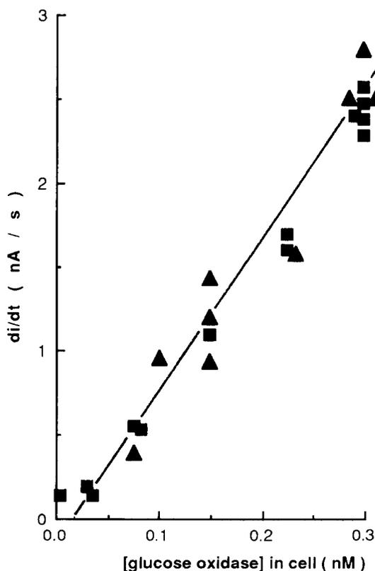
Fig. 6. The dependence of the initial value of  $di/dt$  on the concentration of glucose oxidase (■) and glucose oxidase conjugate (▲) (polarizing potential, 0.4 V; glucose concentration, 30 mM).
