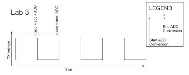
In lab 3, you generated a square wave, and demodulated on the same phase and frequency as the transmitted square wave.
