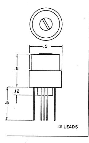
No. 1490 Sensor may be operated from input voltage of 5 to 20 volts DC with 8 to 13 recommended. Input should be both "spike" and polarity protected. Power requirement is approximately 30 mils (0.030 amps).
